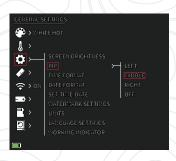
The user has the option to place the PIP window in the upper left/middle/right area of the display.
