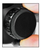
To install a new battery, simply unscrew the battery cap on the rotary switch and install the new battery flat side (+) up.lt is advisable to remove the battery for long-term storage (over a month).
