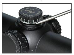
3. Keeping firm grip on the knob, use the pen to turn the dial back to zero, lining up the number zero with the white indicator dot. Only the numbered dial should move – do not allow the entire knob to move or else you will alter your windage and elevation zero settings.
