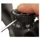
your custom knob about a half-turn counterclockwise and then clockwise back to your sight-in distance to get a feel for the amount of resistance to turn the clicker. If you desire more or less resistance, loosen the three set screws and apply more or less downward pressure onto the custom knob; retighten the set screws. Retest and reset the resistance until satisfied.
