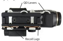
If a lower mounting height is desired, remove the two mounting base screws and QD mount. Remove the mount spacer screws and mount spacer from the sight. Reinstall the QD mount base directly to the sight. Burris recommends using a non-permanent thread locker when reinstalling the mounting base screws.
