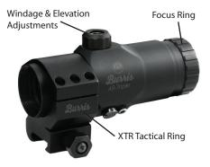
The focus ring at the ocular end of the AR-Tripler is used to focus both the target and the red dot or reticle of the forward sight.Windage and elevation adjustments are provided to center the aiming point and sight picture of the forward optic.Turn these until you have centered the red dot of the forward sight.
