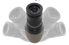
Hold the scope body in place and tighten the thumbscrew by turning to the right or clockwise.
