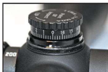
numbered dial should move – do not allow the entire knob to move or else you will alter your windage and elevation zero settings.
