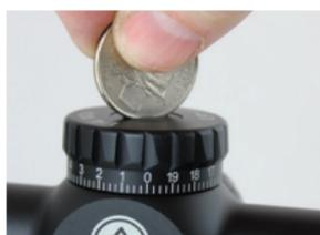
It should rotate freely, and you should not feel or hear any clicks. Rotate the dial until "0" is aligned with the white indicator line.
