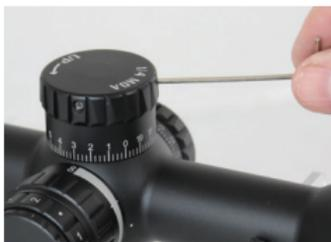
2. Pull up to remove the turret cap. Under the cap is the Zero Click Stop ring with three additional set screws.
