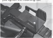
Place the FastFire on the base. Install the provided screws and tighten to 12
