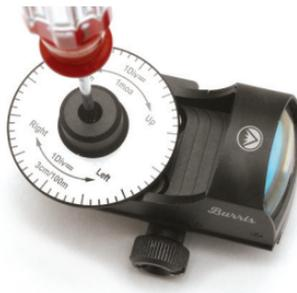
One scale division of this disc (or tick mark) corresponds to 1 minute of angle (MOA), or approximately 1 inch at 100 yards. For other distances, this value is proportional, for example: .5 inch at 50 yards or 0.1 inch at 10 yards. Before shooting, make sure to tighten the lock screws on the rear of the FastFire 2 with the provided screwdriver, making sure not to over-tighten.
