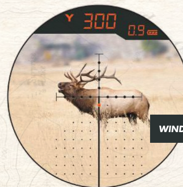
Example 300 yards | 10-mph crosswind shooter holds .9 dots into the wind
